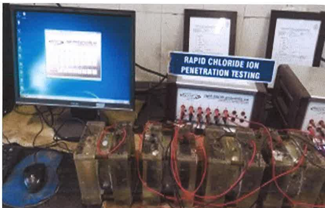
Fig 3: RCPT Test Apparatus
