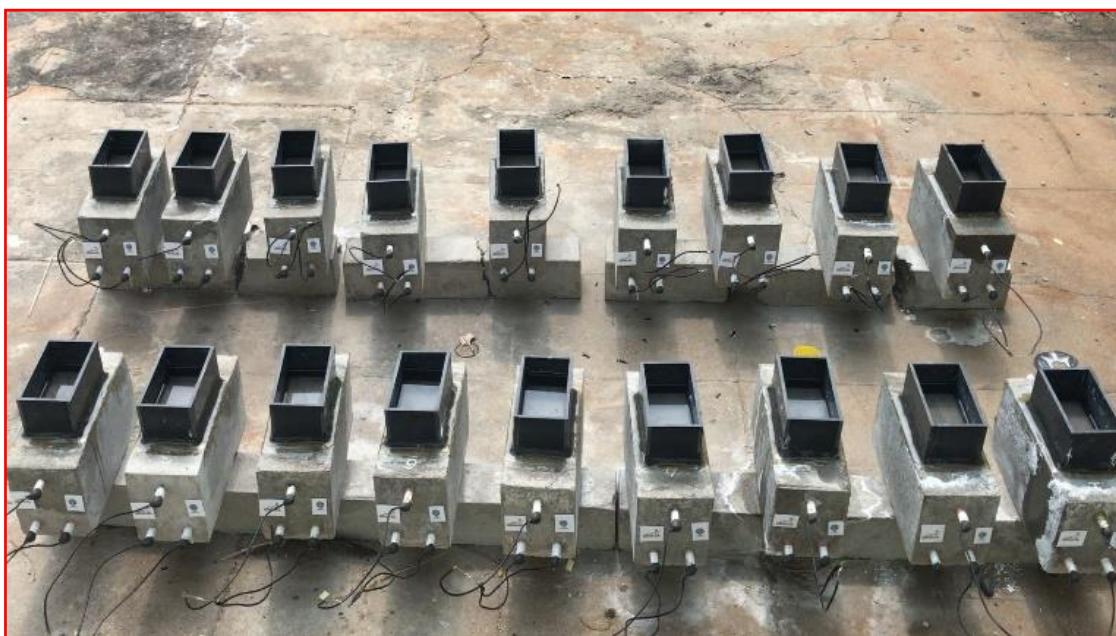
Fig .10 Macrocell specimen exposed at CSIR-CECRI exposure yard
