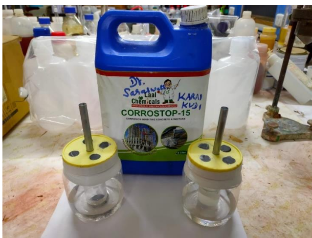
Fig. 4 Test setup for accelerated corrosion test
