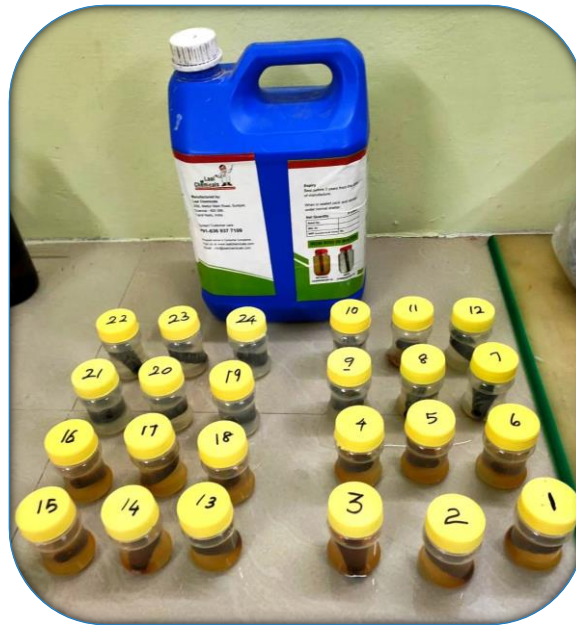
Fig.6 Experimental setup for immersion test
