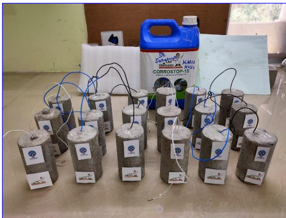
Fig.8 Concrete cylinders for polarization test
