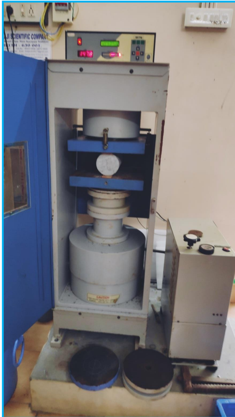
Fig 2. Spiltting tensile strength test is in progress
