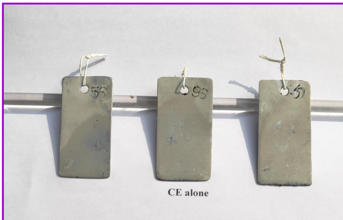
Fig 15 Appearance of test specimen exposed in CE
