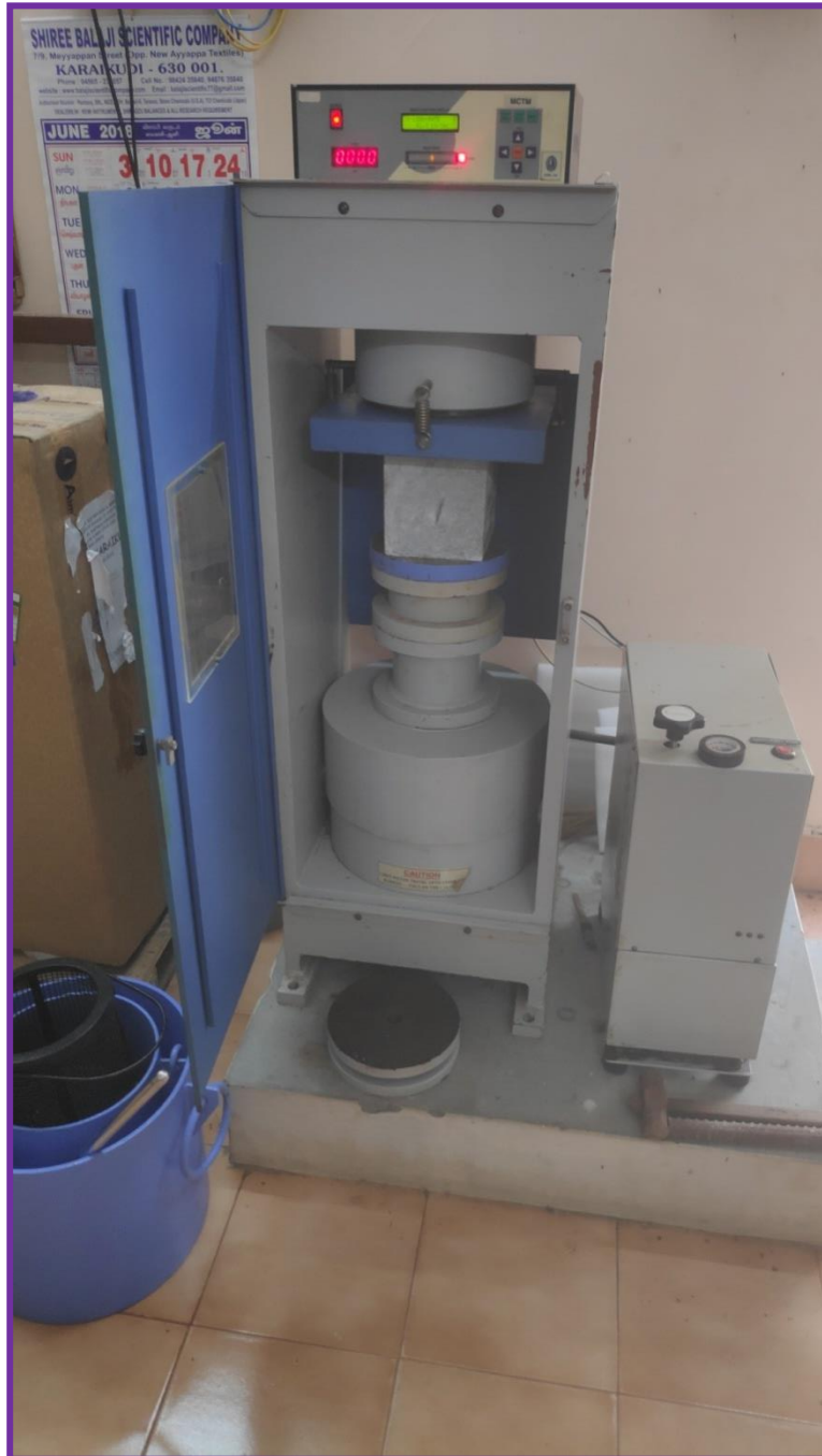
Fig 1. Compressive strength test is in progress
