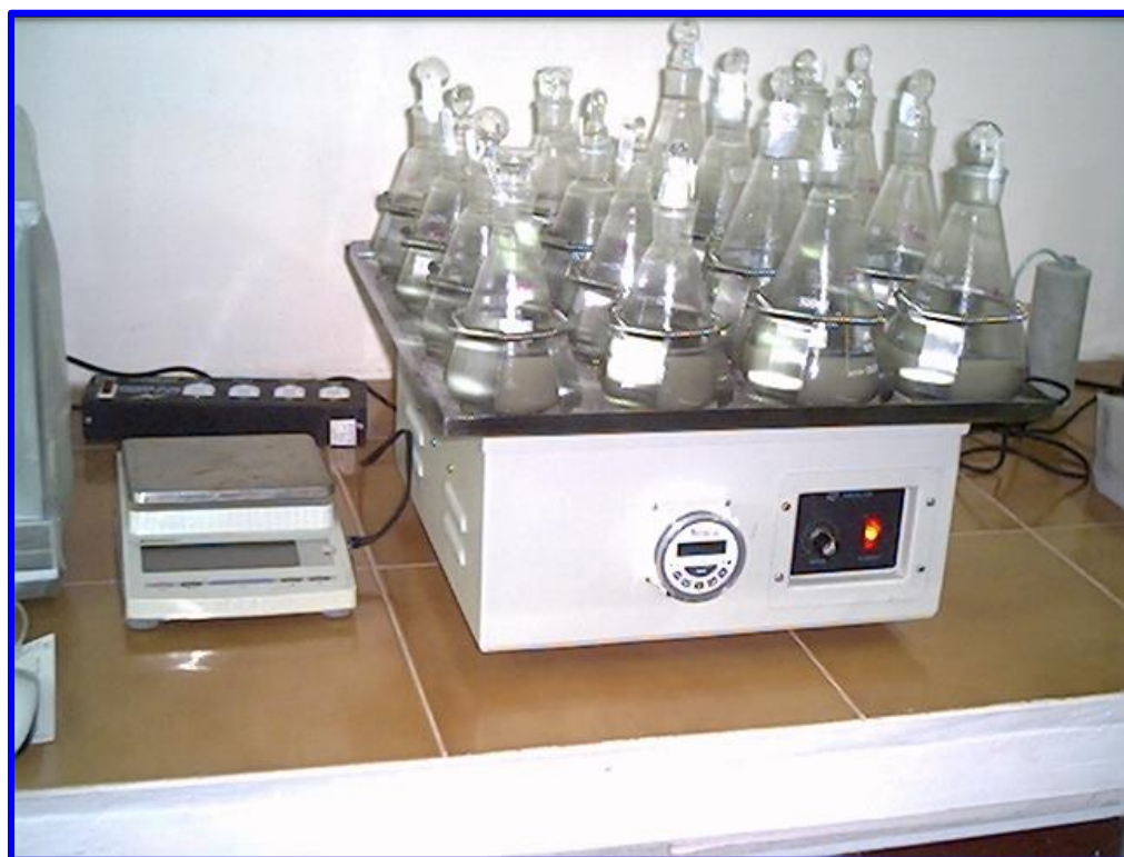
Fig 4 Preparation of cement extract using Digital electronic shaker
